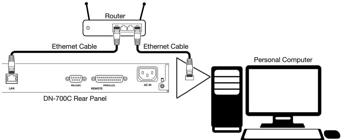
**Note:** Only one network user can be connected to DN-700C at a time. This means that two different computers cannot be used for serial communication with DN-700C at the same time, and you cannot use the LAN port for serial communication while DN-700C is already being controlled by the web browser remote.
