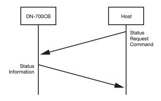
Status information automatically sent to the host when a change is made from DN-700CB
